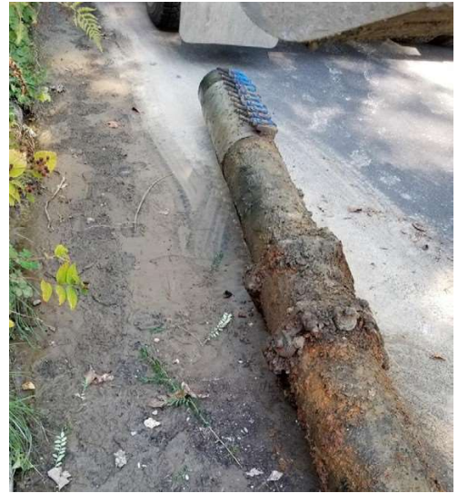
Garden View pipe that was replaced in 2022 shows extensive corrosion.
